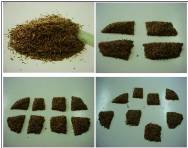
Fig 1: Hand halving method (Image courtesy FAO) 1
